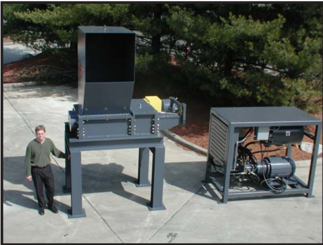
Model HS3632-100 Shown with Enclosed Hopper, Stand and Hydraulic Power Unit
