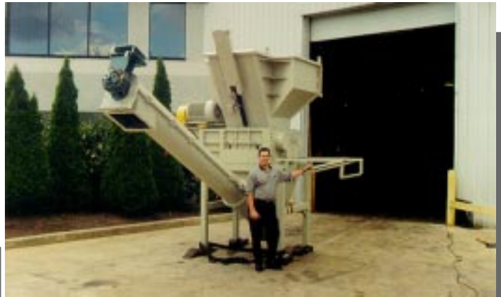
Quad medical waste shredder with infeed ram & output conveyor.
