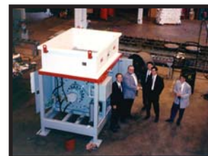
Nan Ya Plastics Corp. in Taipei, Taiwan has a KOMAR auger processor for processing cardboard boxes, pallets and other typical industrial trash for direct feed into their incinerator.
