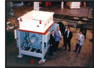
Nan Ya Plastics Corp. in Taipei, Taiwan has a KOMAR auger processor for processing cardboard boxes, pallets and other typical industrial trash for direct feed into their incinerator.
