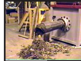
Model HFD-1-75 with water cooled tube and guillotine isolation gate
